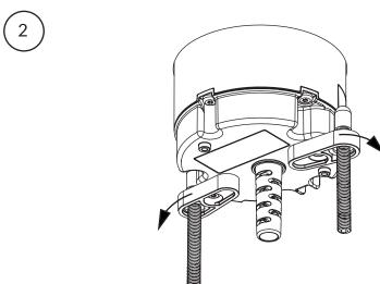
Once located in hole, swivel "wings" out until they've popped into position.
